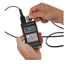
5. While maintaining probe contact with the Test Plate, press the Probe Zero key. The display will show "Prb0" while the Gauge calculates its zero point.
